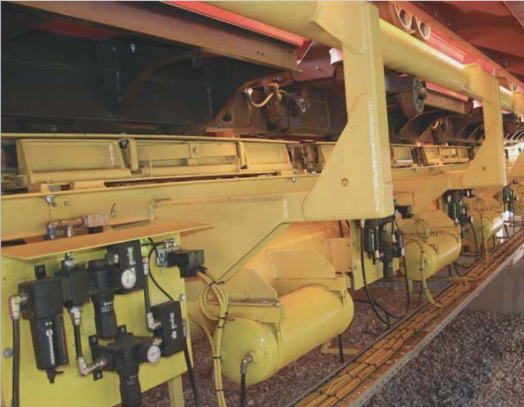
**The air brakes that bring the cars smoothly and safely to a stop**
