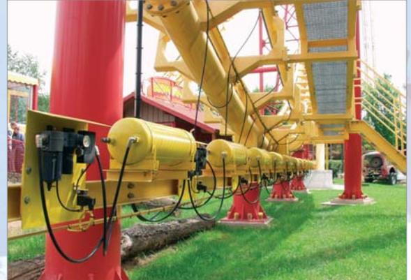
**Storage tanks for the air brakes**
