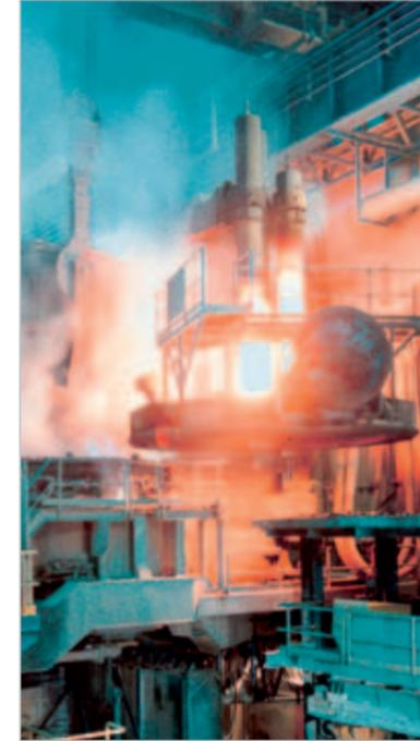
*Carbon electrodes at work in a furnace*
