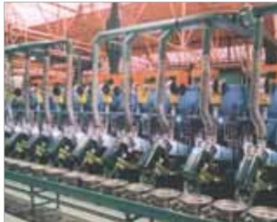
Discs and rims are being welded together
