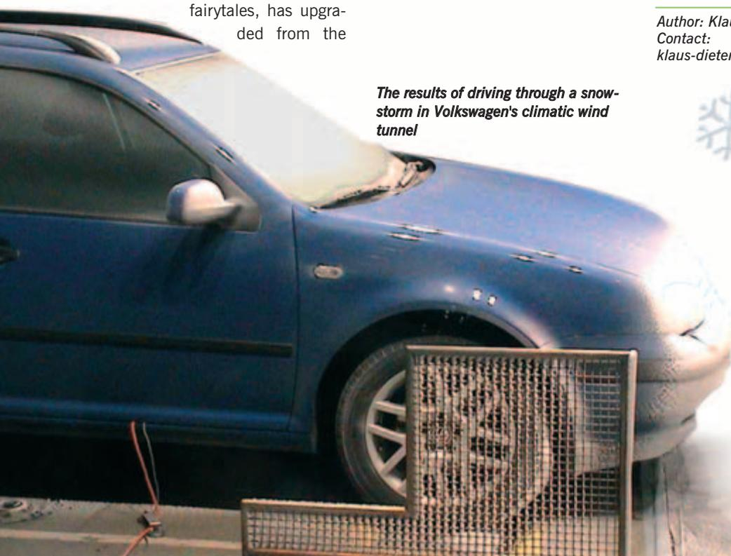
*The results of driving through a snowstorm in Volkswagen's climatic wind tunnel*
