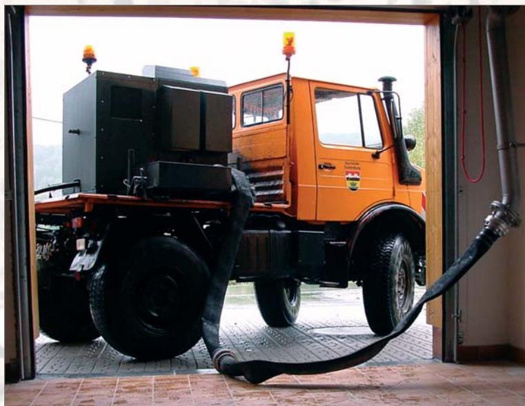
*Air connection fittings are the only modification needed to the treatment plant to enable the use of mobile back flushing*
