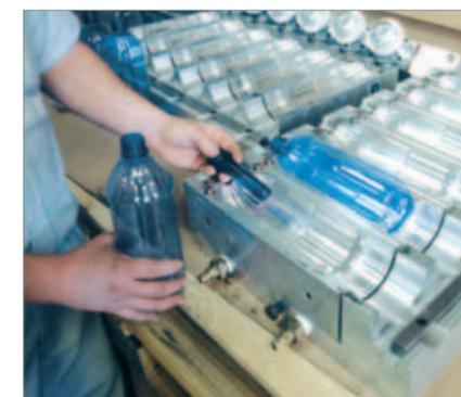
The moulds with air inlets
